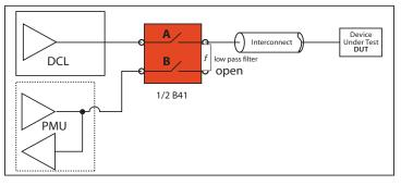
Figure 6: Simplified diagram of PMU/DCL switching circuitry
