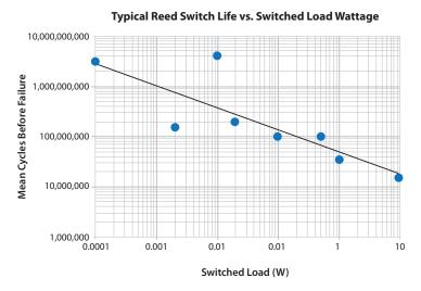
Figure 1: Reed contact life vs. switched wattage
