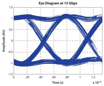
Figure 4: B41 relay eye diagram at 15 Gbps (~10 GHz), CJTPAT bit stream
