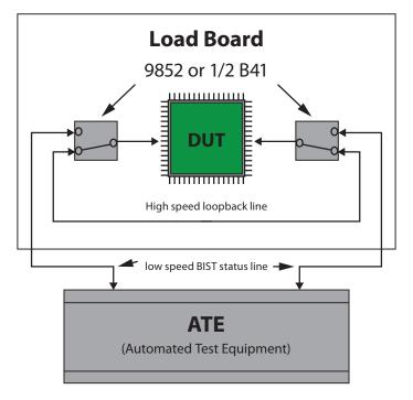
Figure 7: Simplified diagram of loopback testing
