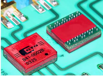
Figure 2: B41 4-channel RF relay showing ball grid array
