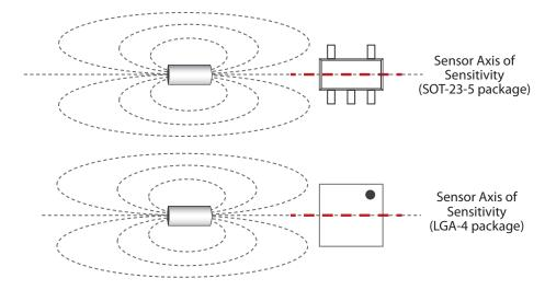
**Note:** The most straightforward way of aligning a magnet with a TMR sensor is by lining up the magnet's magnetization axis with the sensor's Axis of Sensitivity (as shown above). However, there are many other alignments and orientations that will also achieve proper operation. For any questions, or to learn more, please contact Coto Technology. For tips on proper magnetic orientation see our Applications Note:
