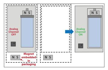
Figure 2 (Left): Portable Liquid level sensing device with magnet embedded in package (Right): Device is removed from packaging, which turns ON the RR142 Analog Channel. From this point onward, the RR142 can detect the position of the magnet mounted on the plunger.
