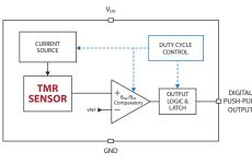
Functional Block Diagram for Analog Channel
