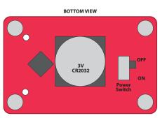
the board correctly in the box, [2] ensure wake-up magnet is present in the box, [3] turn OFF the power switch.
