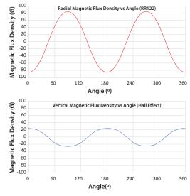
Figure 2: Comparison of Magnetic Flux Density vs. Angle
