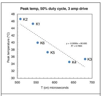
Fig. 1 Peak temperature of six CS128 relays vs. measured turnon time.
