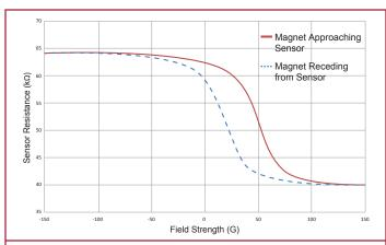
The magnetic sensitivity transfer curve illustrates the characteristic behavior of an analog TMR sensor's resistance change as the strength of an applied magnetic field changes.
