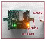
When a sufficiently strong magnetic field is presented to the RR130 on the right side of the board, it will toggle a yellow LED on.
