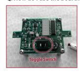
A. There is a toggle switch located near the bottom center of the board. Toggling the switch to the left will turn the board "on" with visual feedback only. Toggling the switch to the right will turn it "on" with both audio and visual feedback active.
