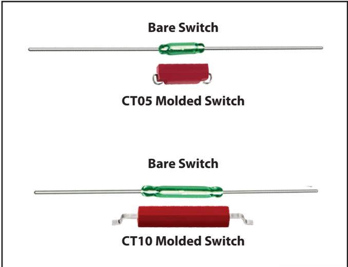
**Fig. 4** bare glass reed switches are fragile, and a better choice is a plastic encapsulated reed switch such as Coto Technology's CT05 or CT10 series. They consist of a high-quality reed switch encapsulated in a hard epoxy resin, which effectively "splints" the reed switch, protecting it from shock, vibration and environmental damage.
