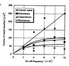
Fig. 6. Dependence of the volume of bumps of transferred Ru metal on R.C.L and coaxial cable as circuit loads as a function of on/off frequencies.
