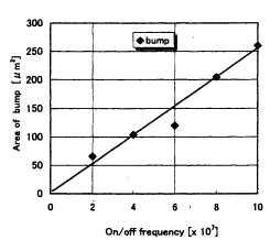
Fig. 2. Bump areas for transferred Rh 1 metal plotted against on/off frequencies.
