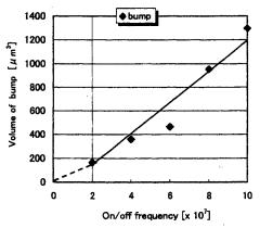
Fig. 3 Bump volumes of transferred Rh 1 metal plotted against on/off frequencies.
