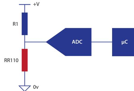
Figure 2: Simple RR110 output measurement with ADC
