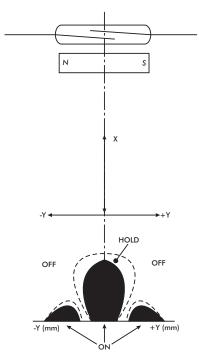
13.1: Movement, with the magnetic field parallel to the dry-reed switch
