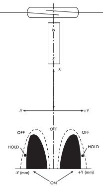
13.3: Movement, with the magnetic field perpendicular to the dry-reed switch
