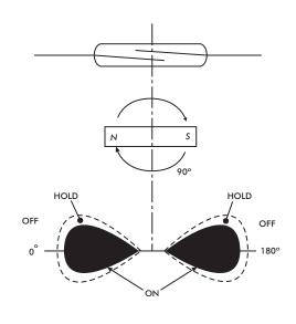
13.2: Rotational movement with a bar shaped permanent magnet
