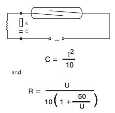
where: C in  $\mu$ F; I in A; R in  $\Omega$ ; U in V.
