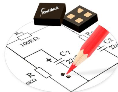
Coto Technology's RedRock RR121 digital sensor, a TMR-based solution that incorporates a tiny LGA-4 package with high magnetic sensitivity and low power consumption. RedRock is immune to cold welding from long periods of contact closure and consumes very low power, all in a package only 0.45mm high with a 1.4 x 1.4mm<sup>2</sup> footprint.
