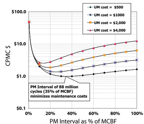
For a full description of the methods used to calculate the Weibull statistics and the CPMC minimization algorithm, take a look at a White Paper called "Testing Reed Switches and Relays for Reliability," available on the Coto Website.
